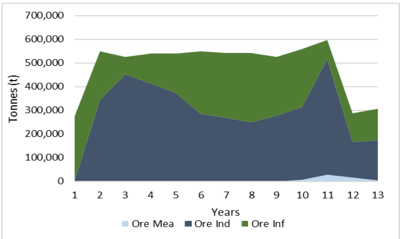
Figure 32 – LOM schedule of Annual Tonnes at various MRE categories on a year by year basis.
